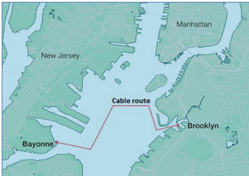
**The cable route of the ABB 345 kV cable system, with the southern tip of Manhattan in the top right-hand corner. The indirect route is due to the many shipping channels and anchorage areas in the busy harbor waters.**
